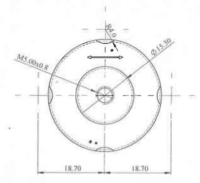
Note: Unspecified linear tolerance is  $\pm 0.05$ Angular tolerance is  $\pm 0^{\circ}15'$
